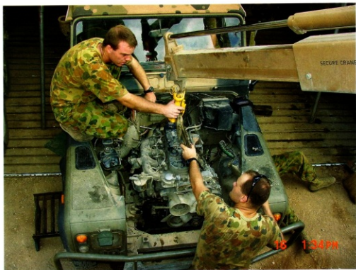
CPL McAnlay and CFN Dare replace an engine in a Land Rover after replacing the clutch.
