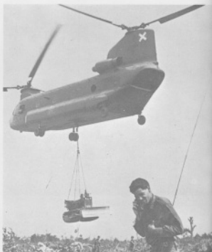
A Chinook helicopter lifts a bulldozer from a fire support base.
